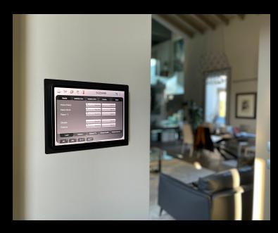
Therefore, the implemented solution provided with simple interfaces for single commands with the Bticino MyHome keypads, advanced interfaces for multi-device control such as Vantage Equinox 40 and a unique and fully customizable interface for a complete home control via Lifetronic "Sweet Home for Vantage" application.
