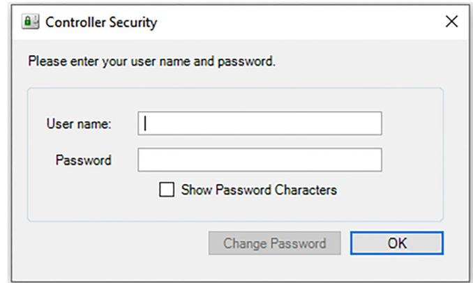
6. With security settings enabled, Design Center will require use of a valid username and password to connect to the controller. When making a new connection, the Controller Security window will appear. Enter either the default username “admin” or “administrator” and the new password you made, or your unique username and password from step 4. Check **Show Password Characters** to verify your password. Select **OK** to log in to the controller.
