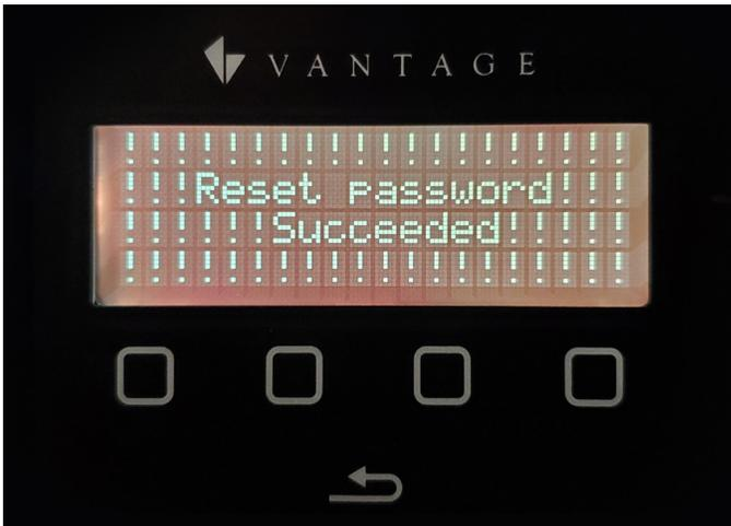
4. A new screen will confirm **Reset password Succeeded!** Tap the exit arrow twice to return to the main screen. Then go to **SECTION TWO** to follow the password setup process.
