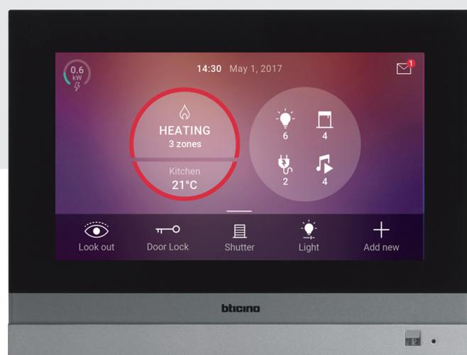
When used as a connected internal unit, **HOMETOUCH** does not require apartment interface item 346850. In case of integration with the **MyHOME\_Up** system, full system supervision is guaranteed without the need of interface item F422.
