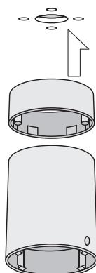
**EN** Secure the mounting box to the ceiling using the holes cut. Then, secure the mounting box to the extender using the supplied fixings.
