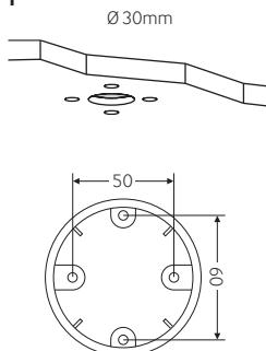
**EN** Cut a 30mm diameter hole in the ceiling for the wires, and mounting holes using the template shown.
