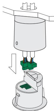
**EN** Wire in plug/s, using wiring diagram on page 2 of the installation guide. Pass the wires through the mounting box and connect the plug/s to the detector.
