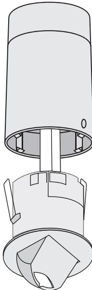
**EN** Bend the springs up and push detector into the mounting box. When fully inserted the springs snap back to hold the device in place.
