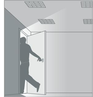
**Presence Detection:** Detectors will switch on lighting automatically when a person enters the room, and switches off lighting automatically when no movement is detected.
