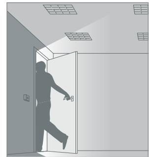
**Absence Detection:** Upon entering the room the person switches on the light as normal, but on leaving the detector switches off the lighting automatically. Lights can also be switched off manually.
